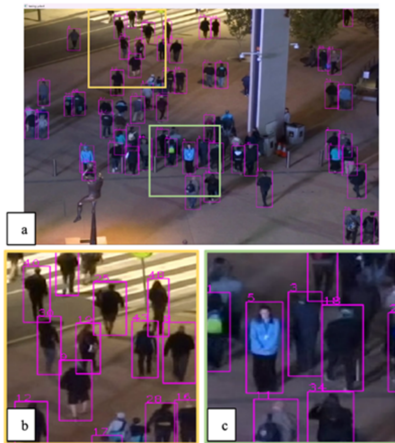
Fig. 1 Sample Output of the YOLOv4+SORT Tracking System: (a) Full-screen output. (b) Magnified yellow box. (c) Magnified green box.
